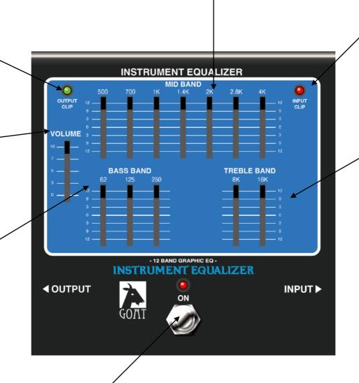
①INPUT CLIP: Monitor with LEDs Monitors the input level of the preamplifier.
